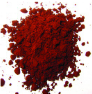
Astaxanthin powder that has not been microencapsulated. This product will not be stable and should not be used for consumer products.
